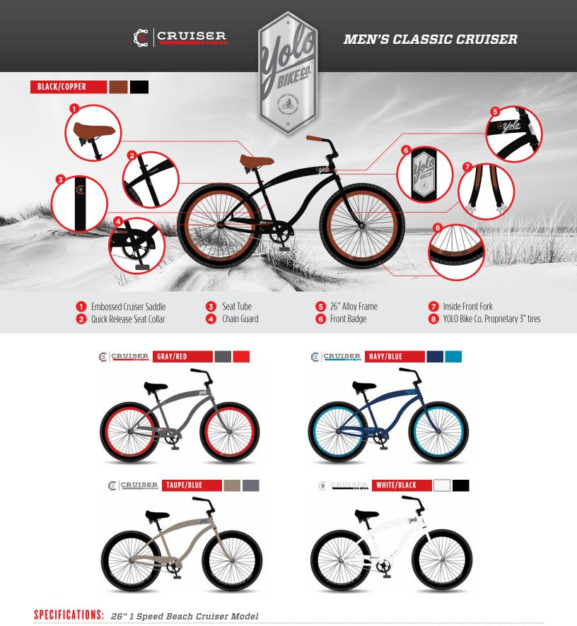
FRAME: 26" Alloy FORK: Steel 1 1/8" HEADSET: 1 1/8" Threadless headset STEM: Alloy 25.4 Clamp Diameter HANDLEBAR: 25.4" Clamp Diameter x 685mm Wide CHAIN: KMC Rust-Buster
